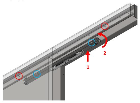
Hang the glass with the opening of the hanger brackets facing away from the pocket as shown. Glass hangs on the round posts circled in blue in the previous image.
